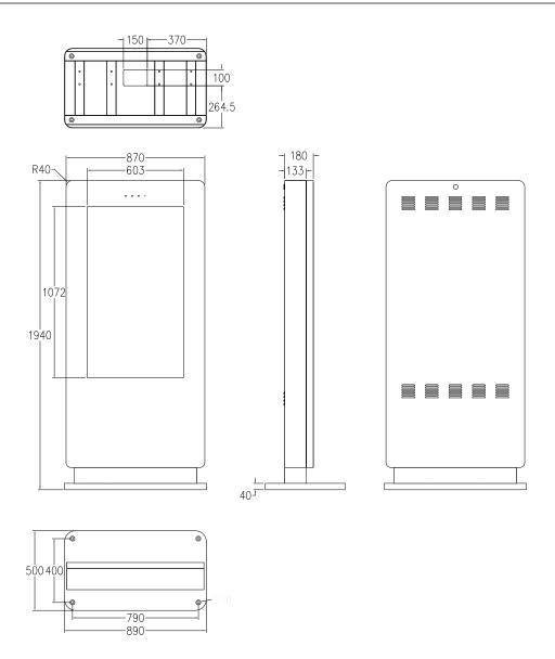
Note: The  $\varnothing 30$  holes are for access, we recommend using M10 anchor bolts that will fit into the  $\varnothing 16$  holes.
