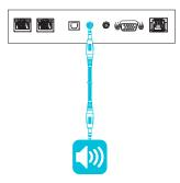
In addition to the stereo 3.5 mm out connector, the display provides a Sony/Philips Digital Interface (S/PDIF) out connector (pictured). S/PDIF is a digital audio transmission medium. You need an audio system that has an S/PDIF input to decode this connection to analog. Most external sound bars include a S/PDIF connector.
