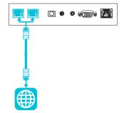
The display requires a network and internet connection for downloading software and firmware updates, and a number of the iQ apps require a network connection as well. You can connect to a network using Wi-Fi or one of the RJ45 jacks.
