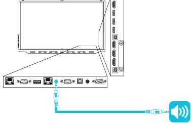
In addition to the stereo 3.5 mm out connector, the display provides a Sony/Philips Digital Interface (S/PDIF) out connector (pictured). S/PDIF is a digital audio transmission medium. You need an audio receiver that supports S/PDIF to decode this connection to analog for use with an external sound bar or other audio system.
