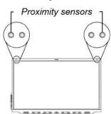
The proximity sensors are located in the top-left and top-right corners of the display's frame.
