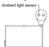
The ambient light sensor is located in the top-right corner of the display's frame.
